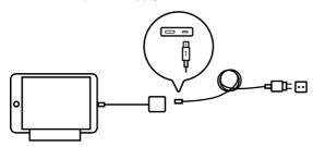
4. Connect the connector cable (20 cm) to the USB hub.
