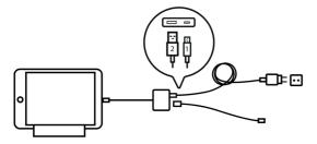
5. Turn on the tablet and follow the on-screen instructions. The tablet is ready to be connected with the recorder.
